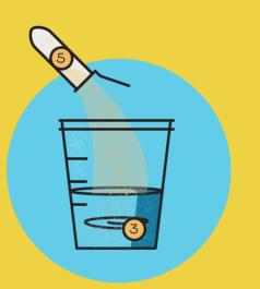
Pour 80 ml of water into the measuring cup (3) and pour in the entire contents of the citric acid capsule (5).
